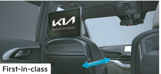
Rear Seat Entertainment Screen and Walk-in Lever
